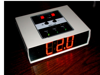
C. Continue pressing timer-3, then release RESET button. The display will show SEL to signify "Mode Select".
